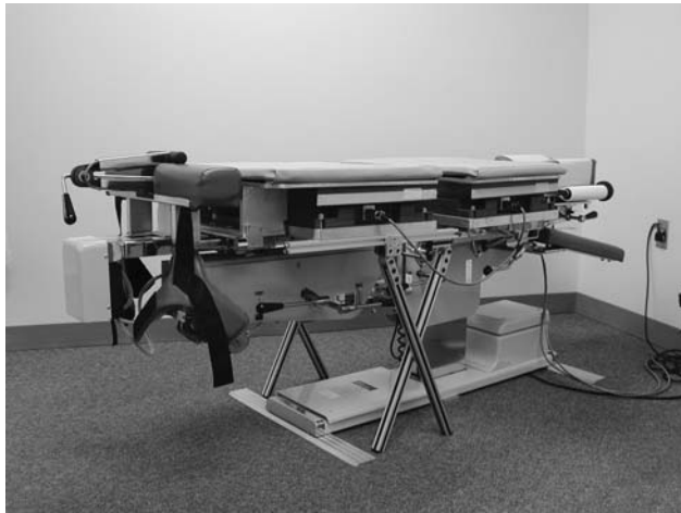
FIG. 1. Flexion–distraction table with force plates installed in the thoracic and pelvic sections.
